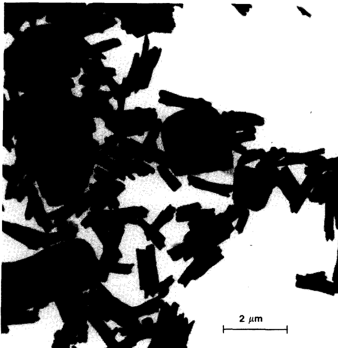
FIG. 6. STEM picture of \text{MoO}_3\text{-BiPO}_4 (1:1) prepared by dispersion-freeze-drying in n -pentane.
