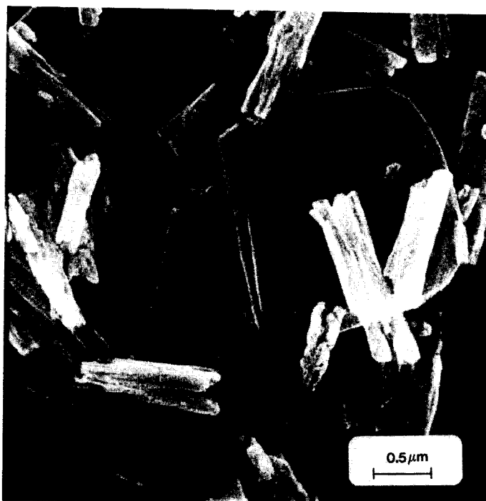
FIG. 7. SEM picture of \text{MoO}_3\text{-BiPO}_4 (1 : 1) prepared in dispersion-freeze-drying in n -pentane.
